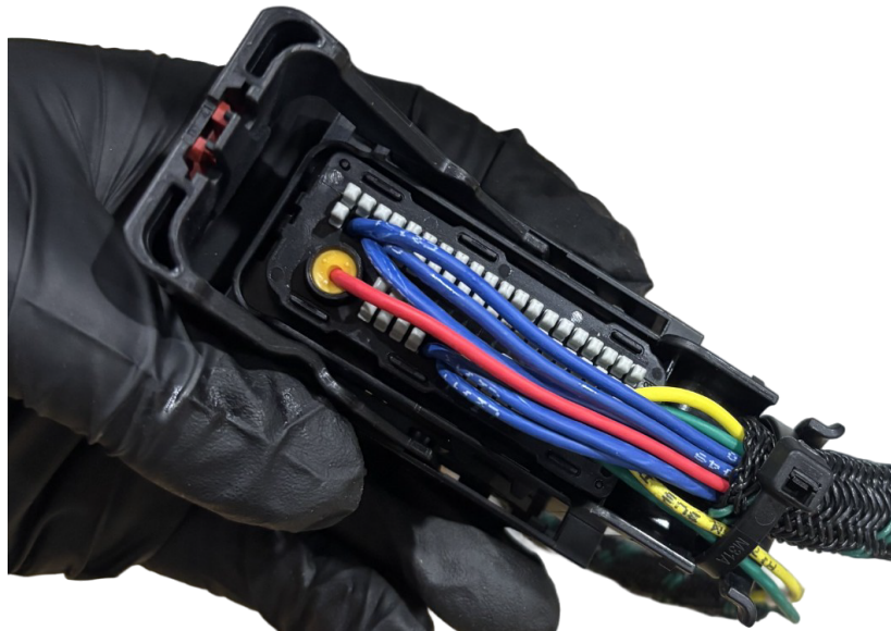
Figure 23 – Securing C2 Connector Harness
